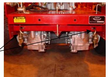
Hydro system by-pass release pins allow the wheels to spin freely (pull out and detent two pins for free wheeling).
